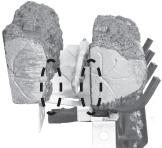
Ensure the rear and front logs are snug up against the main burner bracket.
