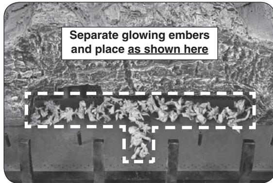
Separate a portion of the glowing embers into small pieces and evenly place them along the rear and center burner ports as shown.
