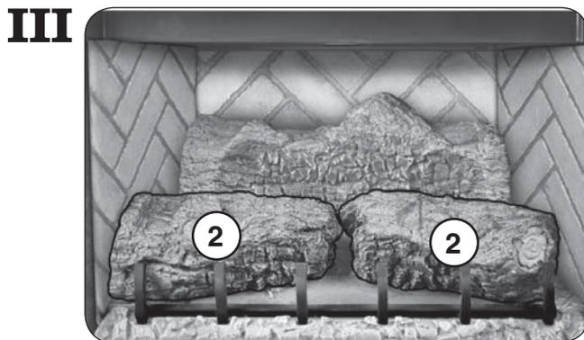
Place the left and right front log pieces (log #2) as shown. The bottom of the logs each have two holes that align with the pegs found on the burner.
