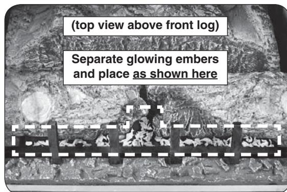
Separate the remaining glowing embers into small pieces and evenly place them along the front and center burner ports as shown.
