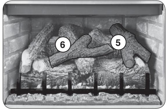
Place the right and middle top logs (logs #5 and #6) as shown. The logs below have notches to aid in positioning the top logs.
