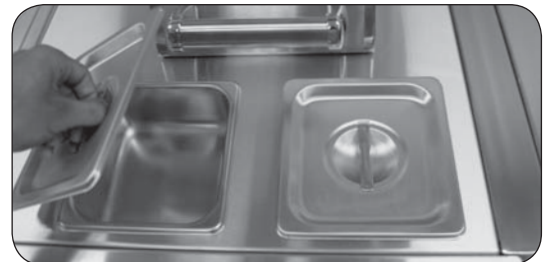
Fig. 6-3 Slide containers into countertop
