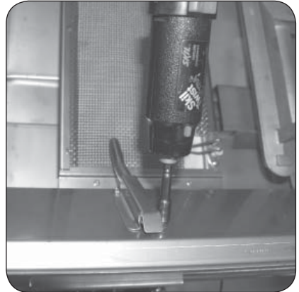
Fig. 4-2 Install new lighting tube
