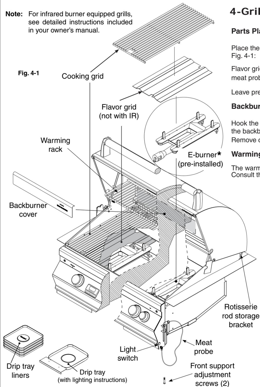
**\* The burner ports and carry-over slots must be kept clean to ensure proper ignition and operation.**
