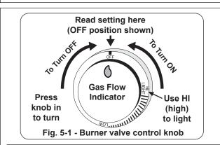
For your convenience and safety; when the control knob is turned to the ON position, the gas flow indicator will change from blue to red. (Red indicates gas flow.) See Fig. 5-1.
