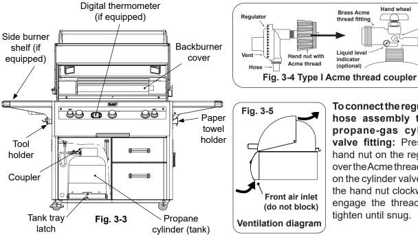
To connect the regulator/ hose assembly to the propane-gas cylinder valve fitting: Press the hand nut on the regulator over the Acme thread fitting on the cylinder valve. Turn the hand nut clockwise to engage the threads and tighten until snug.
