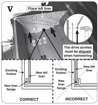
Place the left liner (item 4) as shown above. Rest the liner <a href="OVER">OVER</a> the front and rear liner flanges (hiding the flanges) and ensure the 4 holes are aligned with the 4 grill wall rivets. To secure the liner, align each drive screw (included in kit) with the corresponding hole and carefully hammer each drive screw into the panel. Use needle-nose pliers to assist in holding the drive screws properly.
