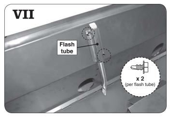
Install the new flash tube by aligning the flash tube over the original liner mounting holes. Using a 1/4" nut driver, affix the flash tube with the supplied hex screws. Repeat this procedure for the other flash tubes.
