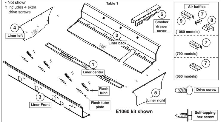
This firebox liner kit is for installation on Echelon grills. Installation on an E1060 is depicted in this instruction.
