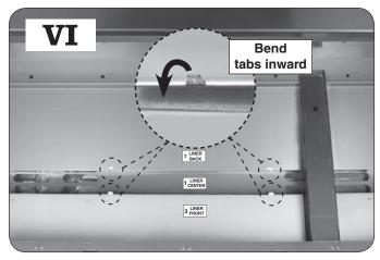
Using pliers, bend in the four tabs inward toward the middle of the center liner to lock the liner panels together.
