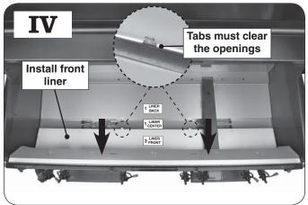
Place the <u>front liner</u> (item 3) ensuring it rests flat against the grill <u>front firebox wall</u>, and the two tabs (on center liner) extend up through the slots in the front liner.
