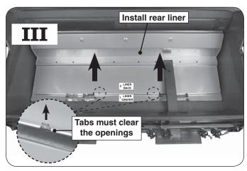
Place the <u>rear liner</u> (item 2) ensuring it rests flat against grill <u>rear firebox wall</u>. The two tabs (on center liner) must extend up through the slots in the rear liner.
