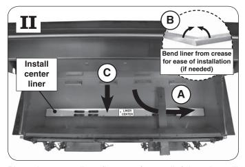
Place the center liner (item 1 of parts list) into the grill drainage channel (A). The liner will need to be bent in order to slide it under the smoker drawer (B). Ensure the liner rests flat in place (C).
