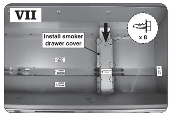
Pre-drill pilot holes through the original grill liner using the supplied drill bits. Place the <u>smoker drawer cover</u> (item 6) ensuring it rests flat on the original smoker drawer. Fasten using the provided self-tapping hex screws and a <sup>1</sup>/<sub>4</sub>" nut driver or equivalent.
