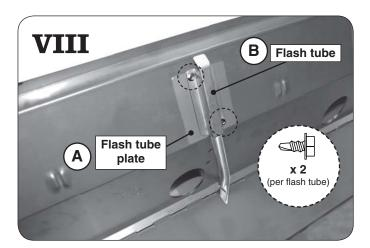
Install the provided flash tube and flash tube plate by aligning the plate (A) and flash tube (B) to the original liner mounting holes. Using a 1/4" nut driver or equivalent, affix with the supplied hex screws. Repeat this procedure for the other flash tubes.
