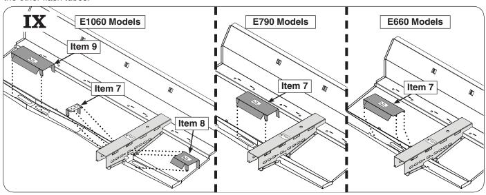
Install the air baffles according to your model above. To properly install, the tabs must slide into the slots located on the liners.
