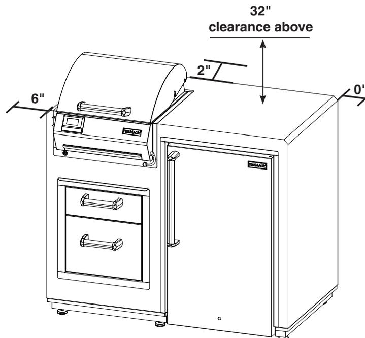
**Floor must be a hard, level surface. Combustible materials permitted.**
