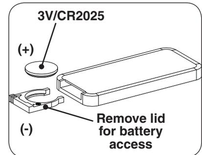
Fig. 10-1 Transmitter battery
