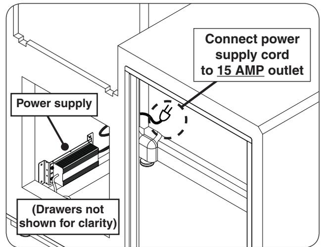
Fig. 8-2 Connect power supply
