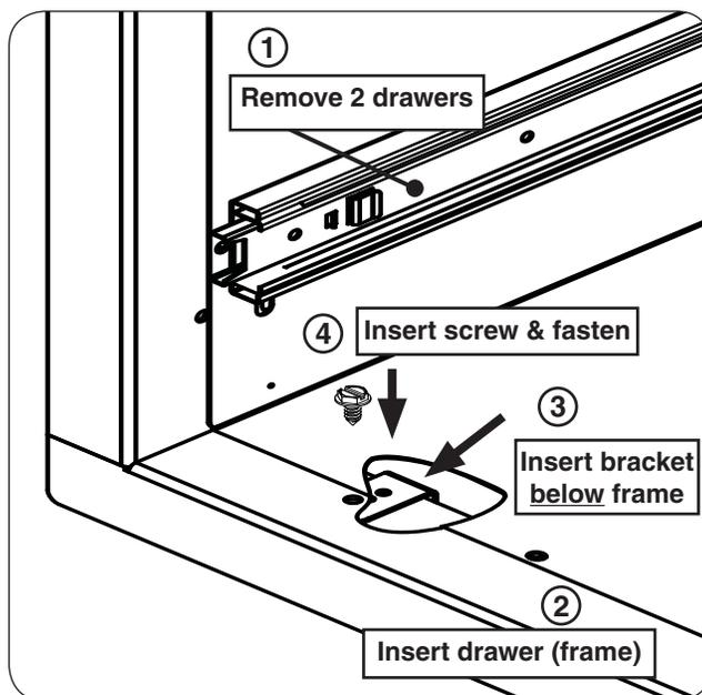
**Fig. 7-3** Install drawer detail
