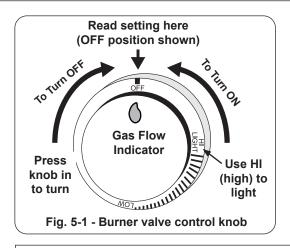
For your convenience and safety; when the control knob is turned to the ON position, the gas flow indicator will change from blue to red. (Red indicates gas flow.) See Fig. 5-1.
