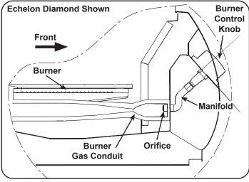
Fig. 3-3 Orifice location cut away side view
