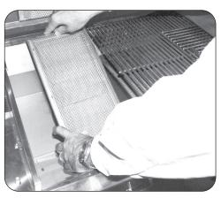
Fig. 6-2 Install new burner
