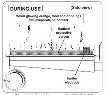
Fig. 8-3 Infrared burner - DURING USE
