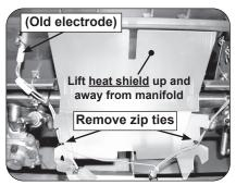
Fig. 2-5 Remove heat shield
