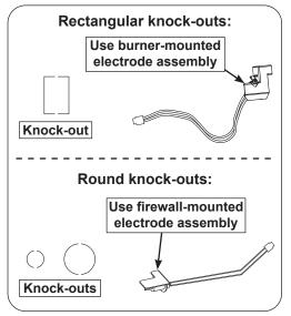
Fig. 3-5 Electrode assembly Identification
