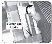
Fig. 2-2 Remove the burner
