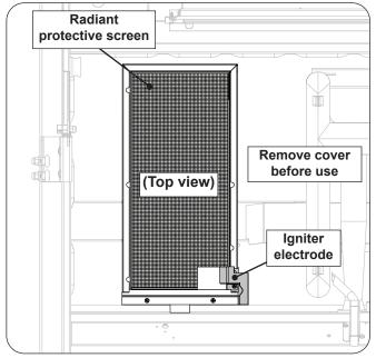
Fig. 8-1 Infrared burner overview
