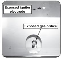
Fig. 3-1 Locate the gas orifice
