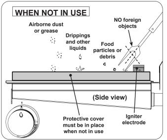
Fig. 8-2 Infrared burner - WHEN NOT IN USE
