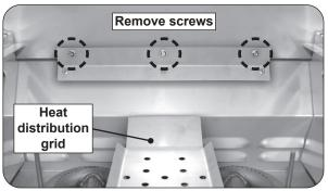
Fig. 2-2 Remove hood - inner screws
