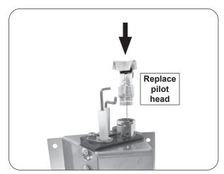
Fig. 3-2 Replace pilot head
