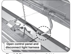
Fig. 1-2 Disconnect oven light harness
