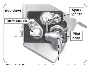
Fig. 3-3 Ensure pilot head properly aligned
