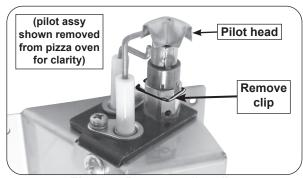
Fig. 2-4 Remove pilot clip
