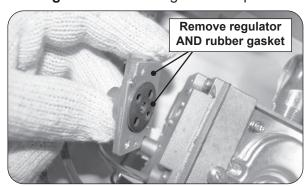
Fig. 4-5 Remove old regulator adapter
