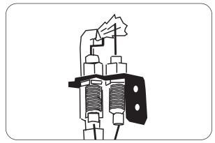
Fig. 6-1 Proper pilot appearance
