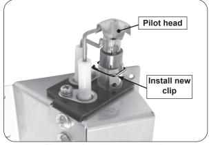
Fig. 3-4 Install new pilot clip
