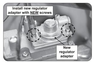
Fig. 5-2 Fasten new regulator adapter
