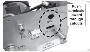
Fig. 4-2 Insert terminals into box
