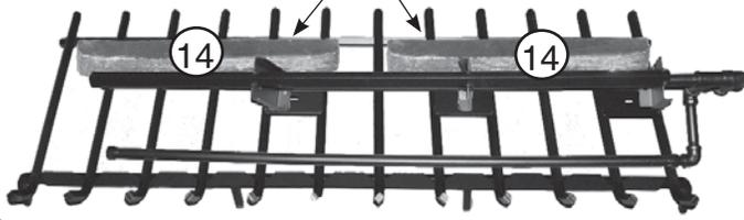
Place the burner system and rear spacer logs
