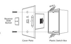
**NOTE:** The remote receiver will only respond to the transmitter when the 3-position slide button on the remote receiver is in the REMOTE position. If the system does not respond to the battery transmitter on initial use, see LEARNING TRANSMITTER TO RECEIVER, and recheck battery positions in the remote receiver.
