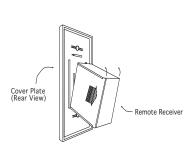
To attach Cover Plate to Receiver box: Position the receiver as shown in diagram to the left with lower tab on cover plate inserted into groove of receiver, (Make sure LEARN hole on cover plate properly aligns with remote receiver) Pull receiver up and snap into top tab of cover plate.
