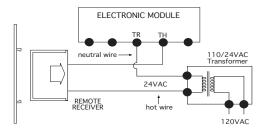
The remote control receiver can be connected, in series, to a 24VAC transformer to the TR (transformer) terminal on the electronic module. Connect the hot wire from the 24VAC transformer to either of the wire terminals on the remote receiver. Connect another wire (included) between the other receiver wire terminal and the TH (thermostat) terminal on the electronic module.
