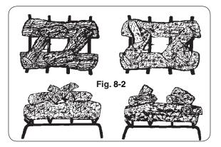
CAUTION: Burn hazard. Logs will remain hot for some time after use. You must maintain the log layout as shown to ensure proper operation of your log set. If you need to reposition any log to maintain the proper layout, use heat-resistant gloves or allow logs adequate time to cool before handling.
