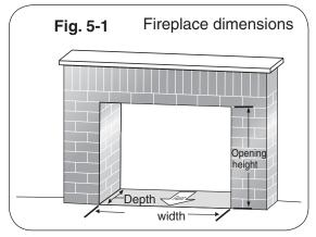
The fireplace must have a gas supply line that has been installed by a qualified technician in accordance with all local codes. The gas supply line must have a ½" minimum interior diameter. If the gas line to the fireplace is longer than 20', a larger diameter line may be necessary.
