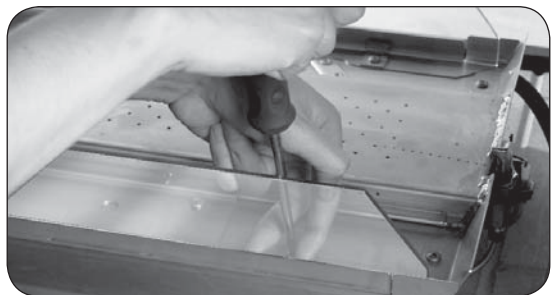
Fig. 10-3 Securing glass panel
