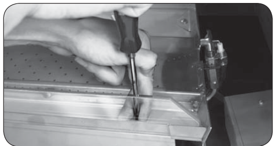
Fig. 10-3 Securing glass panel
