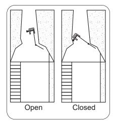
Fig. 6-2 Damper open / closed
