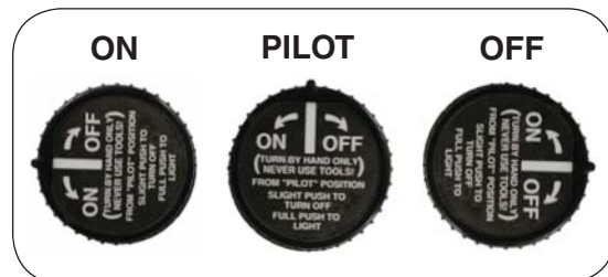
Fig. 17-2 Manual valve operating positions
