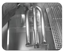
Fig. 1-2 Remove the burner
