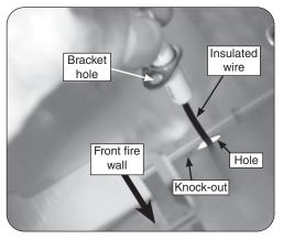
Fig. 3-1 Slide the wire through the fire wall
