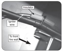
Fig. 3-2 Screw in the new wire insulator
