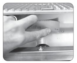
Fig. 4-3 Apply the conversion label
