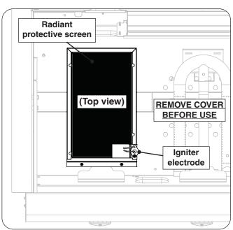
Fig. 5-1 Infrared burner overview
