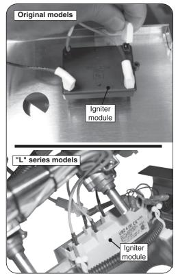
Fig. 2-2 Remove old igniter wire
