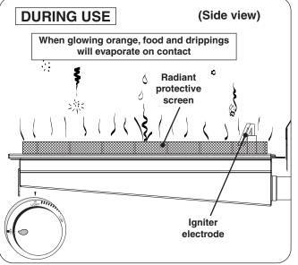
Fig. 5-3 Infrared burner - DURING USE
