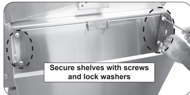
Fig. 13-1 Install folding shelves
