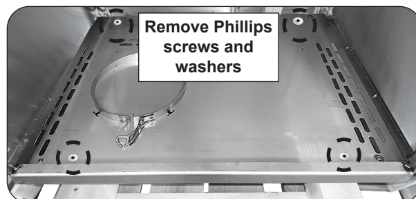
Fig. 9-2 Remove four front screws/washers
