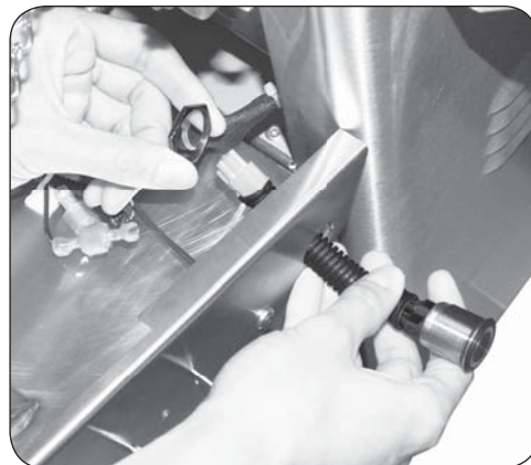
Fig. 2-1 Installing master switch
