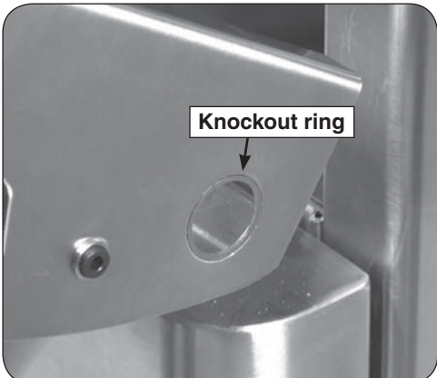
Fig. 1-3 Remove knockout ring (if applicable)
