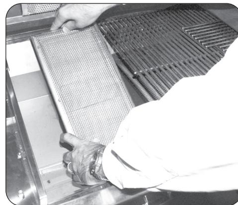
Fig. 4-4 Install new burner
