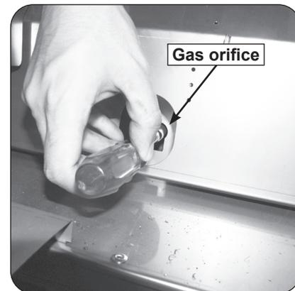
Fig. 3-2 Replace the gas orifice
