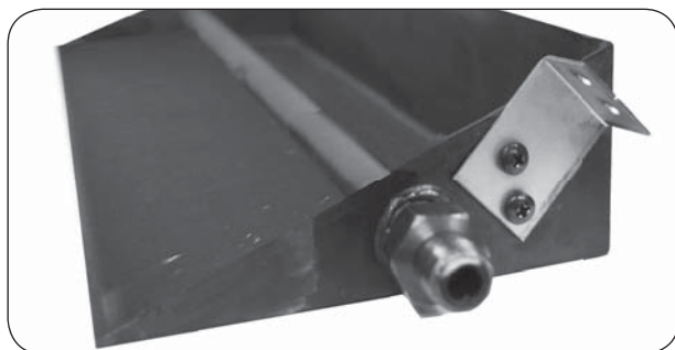
Fig. 7-2 Install pilot bracket
